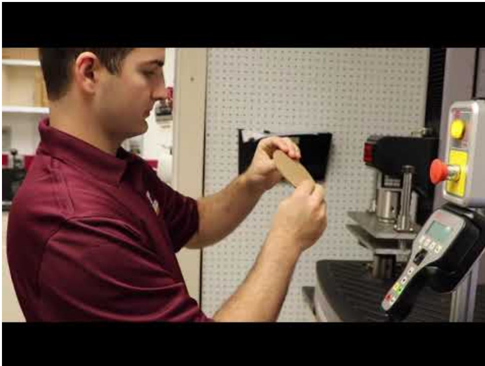
~ Test of the Month: Flat Crush Test ~
